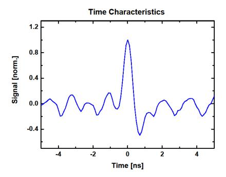
The rise time of the photodetector is defined as the time for the signal to rise from 10% up to 90% of the maximum value.
