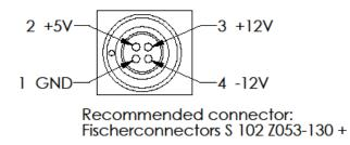
Four pole male connector on detector.
