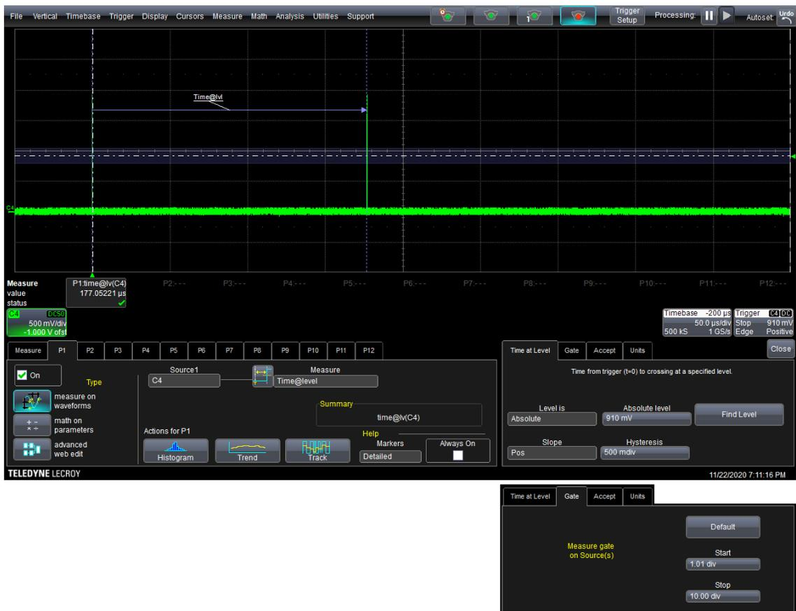
FIG. 5. A measurement is set up on the oscillogram to measure time of a pulse since trigger. A gate is set up to exclude the triggering pulse from the measurement.
