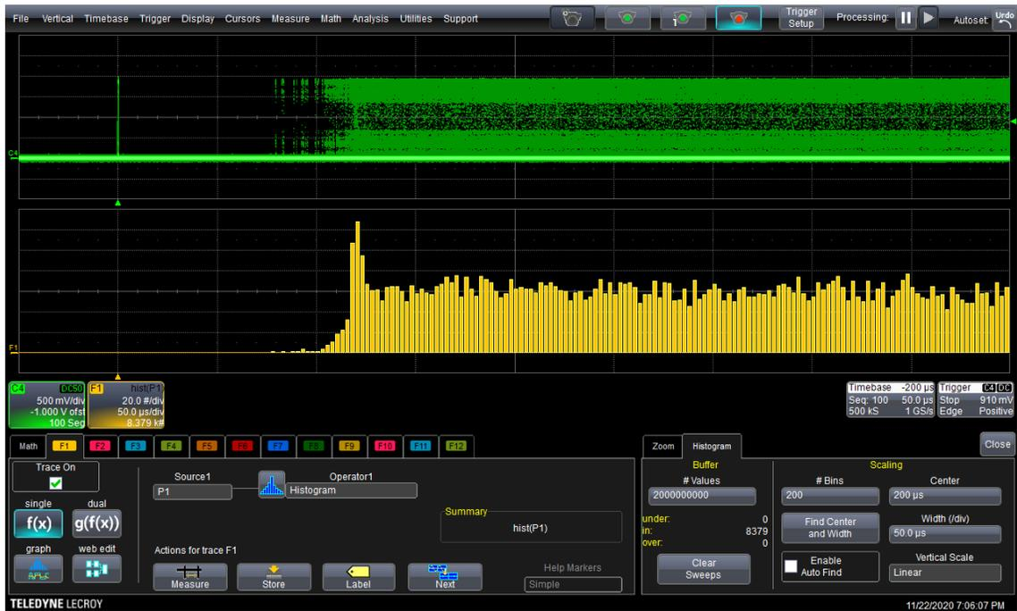
FIG. 6. A histogram of the time measurement shows how the detector recovers from the deadtime. We see a gradual transition from zero to nominal photon detection probability, with a peak in-between that possibly contains afterpulses.
