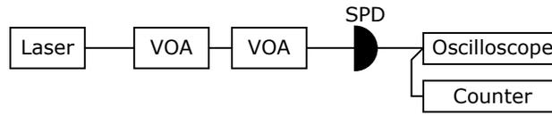
FIG. 7. Suggested setup for measuring photon detection efficiency. VOA, programmable optical attenuator.
