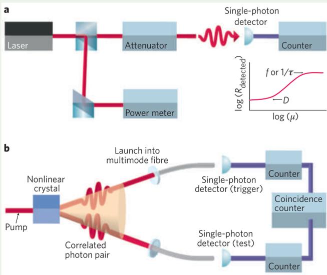
**Figure B1 | Determination of single-photon detector efficiency.**
