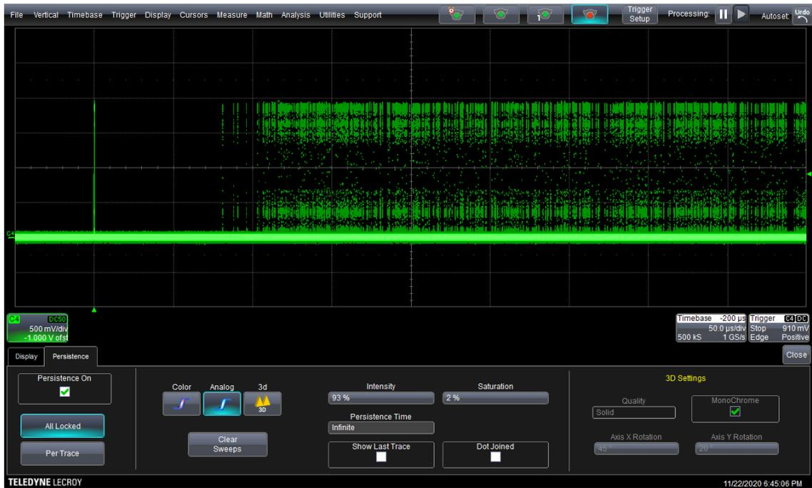
FIG. 4. An example of the oscilloscope screen with an oscillogram of detector output in persistence mode, showing the recovery of sensitivity after a click.
