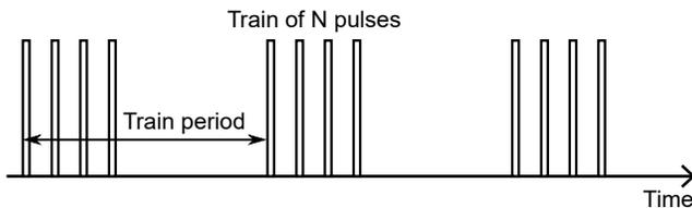
FIG. 1. Trains of laser pulses emitted from QRate laser module.
