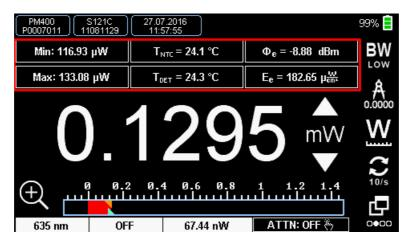
To configure a subpanel, tap to it and select from the drop-down list the desired parameter. Please note, that additional parameters are sensor-dependent, as stated in the table below:
