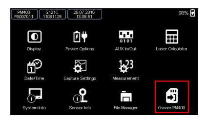
The icon changes to "Owner USB" and an additional red 'memory card' icon **D** appears in the header bar. The connected PC recognizes the PM400 memory as a "Removable Disk" that can be accessed from the Windows explorer:
