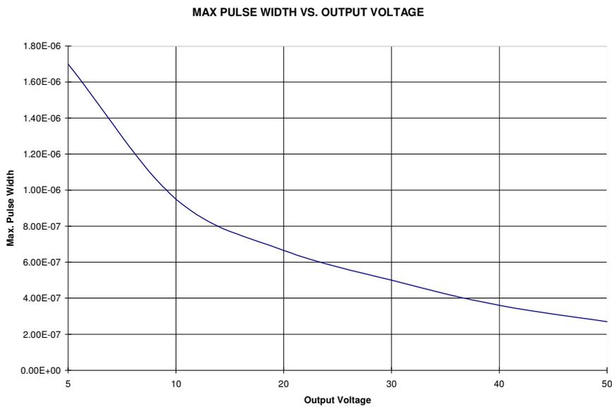
**Figure 14. Pulse width as a function of output**
