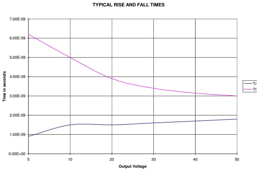
**Figure 16. Pulse rise and fall times**
