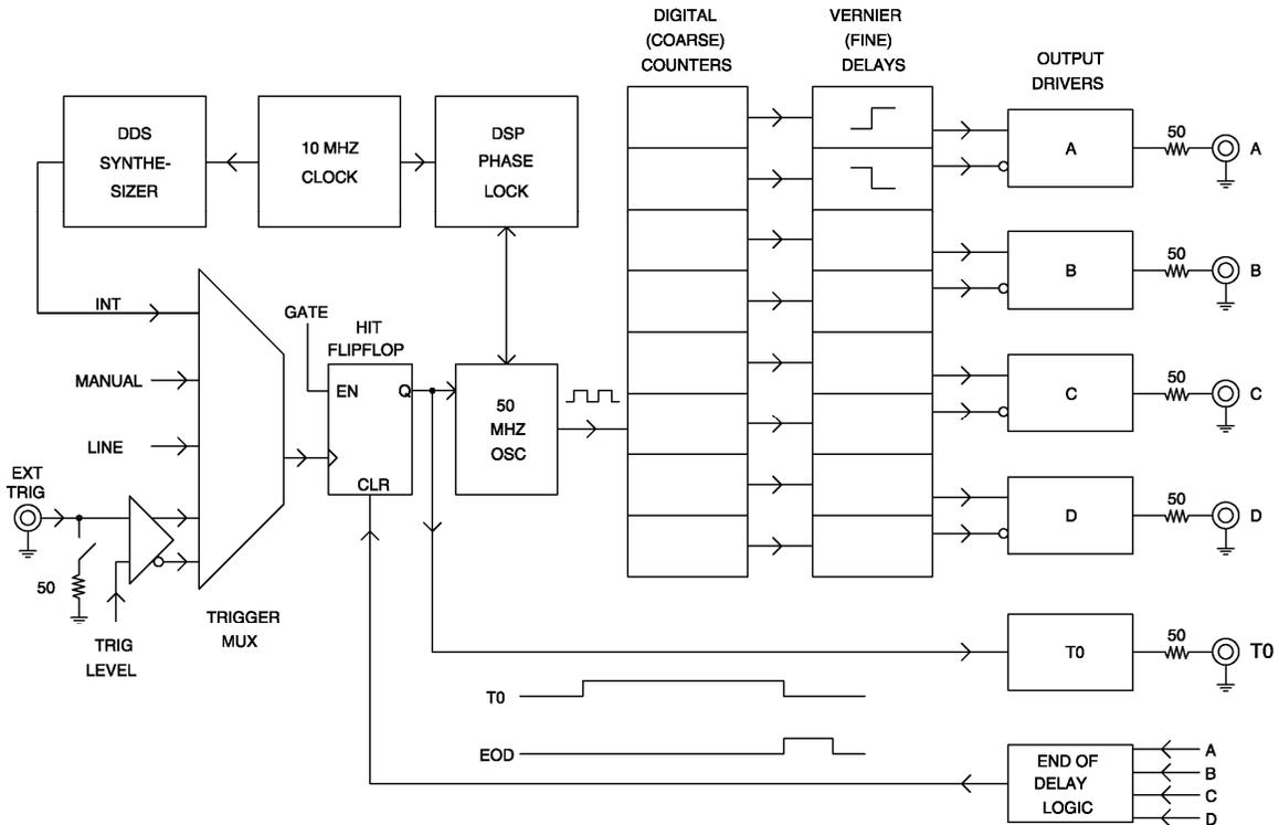
**Figure 2. Block Diagram**
