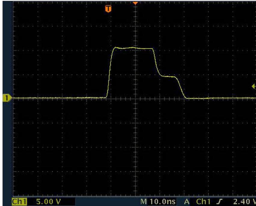
Figure 19. 10 V Pulse with High-Impedance Termination
