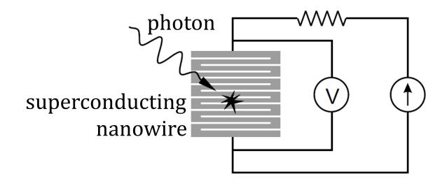
A photon detector is a device that converts a photon into a "click" — a macroscopic pulse of electric current or voltage.
