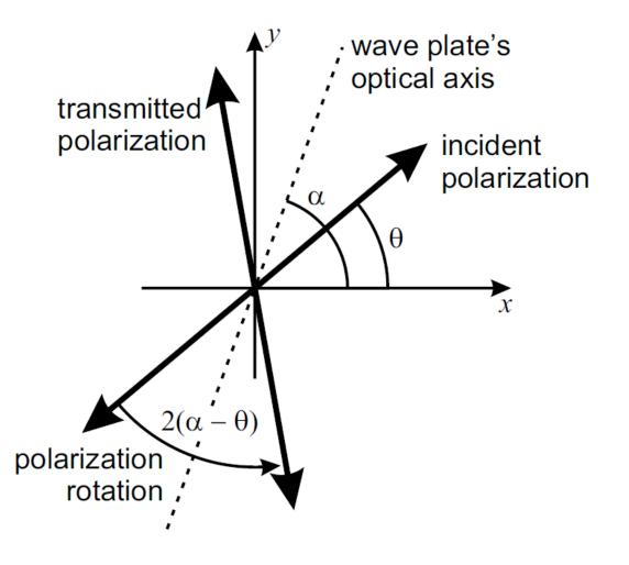
The half-wave plate "flips" the polarization pattern around the vertical (or horizontal) axis akin to a mirror.
