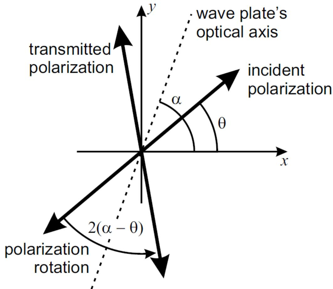
The half-wave plate “flips” the polarization pattern around the vertical (or horizontal) axis akin to a mirror.
