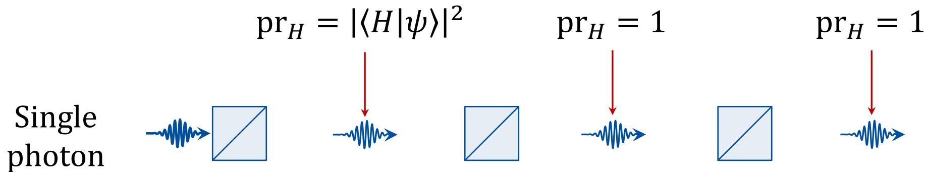
After the PBS, the photon state in the transmitted channel will become  $|H\rangle$ , and in the reflected channel  $|V\rangle$ . If we place a series of additional PBS's in the transmitted channel of the first PBS, the photon will be transmitted through all of these PBS's — there will be no further randomness.
