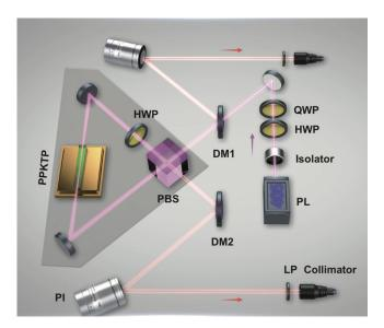
FIG. 20. Schematic of the satellite-borne entangled-photon source. The entangled-photon source in the Micius satellite is based on type-II periodically poled KTiOPO<sub>4</sub> (PPKTP) crystal and the Sagnac interferometer. PL, pump laser; DM, dichromatic mirror; PI, piezoelectric steering mirror; QWP, quarter-wave plate; HWP, half-wave plate; PBS, polarizing beam splitter. From Yin *et al.*, 2017a.
