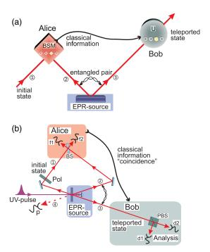
FIG. 4. (a) Principle of quantum teleportation. (b) Setup of the Innsbruck teleportation experiment (Bouwmeester *et al.*, 1997). A pulse of ultraviolet light passing through a nonlinear crystal creates an ancillary pair of entangled photons 2 and 3 in a polarization state  $|\psi^{-}\rangle_{12}$ . The pulse is reflected, and during its second passage through the crystal another pair of photons can be created.
