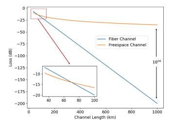
FIG. 10. Typical losses in fiber and free-space channels. The attenuation parameter of fiber is  $\sim$ 0.2 dB/km. The parameters of the free-space channel are based on the design of the Micius satellite. The free-space channel shows an advantage for a distance over  $\sim$ 70 km.
