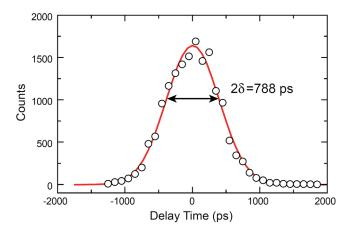
FIG. 17. A typical recorded arrival time of the 1064 nm laser signals at both stations. A synchronization accuracy of 788 ps was observed. From Yin *et al.*, 2012.
