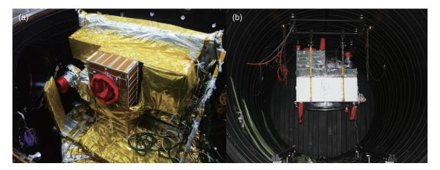
FIG. 21. (a) Thermal-vacuum-optical measurement and (b) thermal balancing testing for a payload combination.
