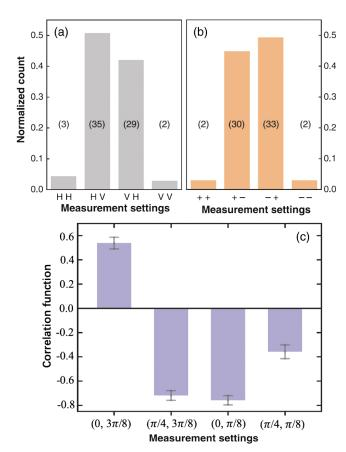
FIG. 32. (a) Normalized two-photon coincidence counts in the measurement setting of the H/V basis. (b) Normalized counts in the diagonal basis. (c) Correlation functions of a Clauser-Horne-Shimony-Holt-type Bell inequality for the entanglement distribution. Error bars are 1 standard deviation and are calculated from propagated Poissonian counting statistics of the raw photon. From Yin *et al.*, 2017a.
