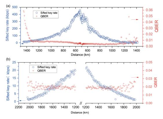
FIG. 30. Performance of high-speed satellite-to-ground QKD. (a) Sifted key rate and observed QBER as a function of physical distance from the satellite to the Nanshan station. (b) Test for long-distance satellite-to-ground QKD. The sifted key rate and observed QBER are at a distance beyond 1200 km. From Chen *et al.*, 2021.
