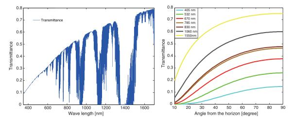
FIG. 11. Simulated atmospheric transmittance for a zenith with different wavelengths (left panel) and different altitude angles (right panel).
