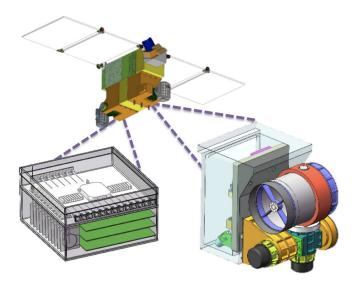
FIG. 44. Preliminary design of small satellites in China. This design will focus on the QKD using downlink channels. The total weight will be less than 100 kg. The orbit height will be 800 km. There will be three or five small quantum satellites for the first step.
