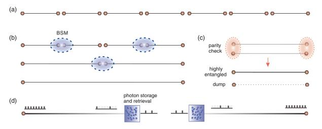
FIG. 8. Principle of quantum repeaters. (a) Dividing the communication channel into *N* segments. (b) Using entanglement swapping to establish entanglement between remote nodes. (c) Using entanglement purification to distill highly entangled pairs between remote nodes. (d) Using quantum memory to store single photons for a sufficiently long time and retrieve the single photon for time synchronized two-photon interference. From Briegel *et al.*, 1998, and Duan *et al.*, 2001.
