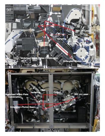
FIG. 19. Top view of a transmitter's optics head. The collimated beam from the entangled-photon source passes through a motorized wave-plate combination and a beam expander and then is combined with the 850 nm synchronization laser using a dichroic mirror. (a) Transmitter 1's optics head. (b) Transmitter 2's optics head. From Liao *et al.*, 2017a.
