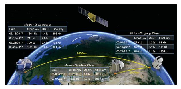
FIG. 36. Illustration of the three cooperating ground stations (Graz, Nanshan, and Xinglong). Listed are all paths used for key generation and the corresponding final key length. From Liao *et al.*, 2018.
