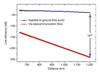
FIG. 29. Link efficiencies for direct transmission through telecommunication optical fibers (red line) and following the satellite-to-ground approach (blue line). The link efficiencies for the latter were calculated by dividing the photon intensity that arrived in front of the detectors at the ground station by that from the output of the satellite's transmitter. From Liao *et al.*, 2017a.
