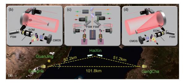
FIG. 15. Bidirectional two-link entanglement distribution over Qinghai Lake at a distance of 101.8 km. From Yin et al., 2012.
