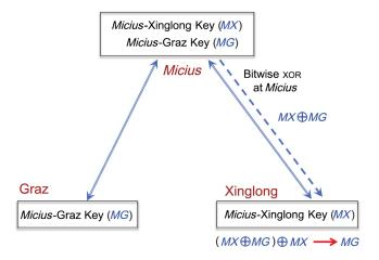
FIG. 37. Schematic of a key exchange procedure between Graz and Xinglong with the satellite as a trusted relay. After Micius distributes a key with Graz (MG) and Xinglong (MX), it performs a bitwise exclusive or operation between those keys (MX  $\oplus$  MG) and sends this combined key via a classical channel toward the Xinglong station. Combining the XORed key at Xinglong with MX leads to the same key (MG) on both sides. From Liao *et al.*, 2018.
