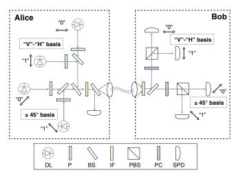
FIG. 6. Polarization optics of the QKD transmitter and receiver. The lasers in the transmitter are attenuated to have an average photon number less than 1. Multidetection events due to the multiphoton component of the weak coherent pulse are recorded but not used for key generation. From Hughes *et al.*, 2002.
