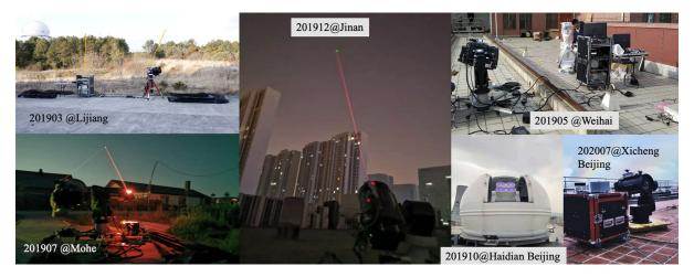
FIG. 45. Experimental demonstration of the feasibility of satellite-to-ground QKD with compact ground stations. By 2020, the QKD with the Micius satellite and the compact ground station had been demonstrated in many Chinese cities, including Beijing, Jinan, Weihai, Lijiang, and Mohe. The typical sifted key rate is ~2 kbits/s.
