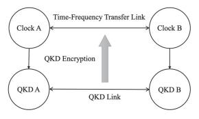
FIG. 49. Diagram of a quantum-secure time-frequency transfer.
