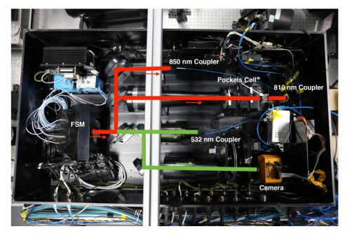
FIG. 24. Photograph of the measurement box at Lijiang station, which represents the typical design of the satellite-based entanglement distribution. From Yin *et al.*, 2017a.
