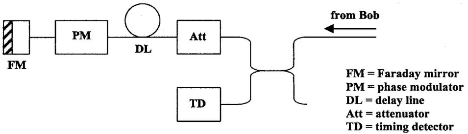
Figure 5. Alice's set-up in the 'plug & play' scheme.
