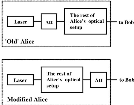
Figure 7. Modification of Alice's set-up.
