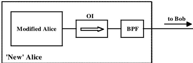
Figure 8. Passive security measures for Alice's set-up.
