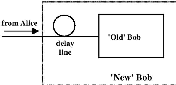
Figure 6. Passive security measures for Bob's set-up.
