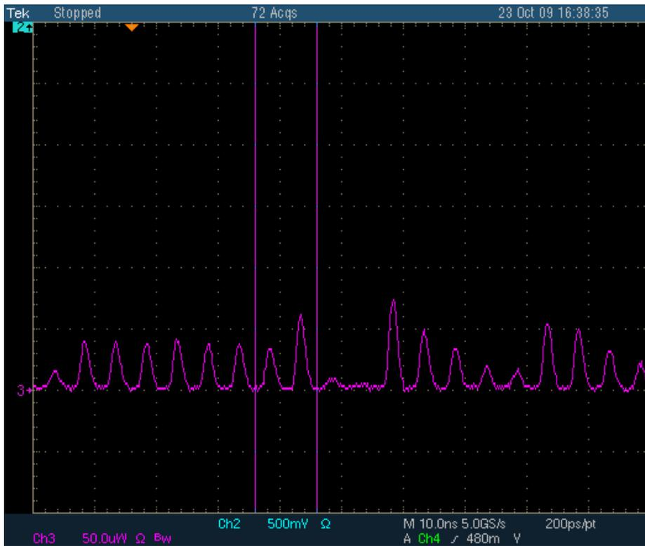
Figure 5.11: Unstable laser pulses
