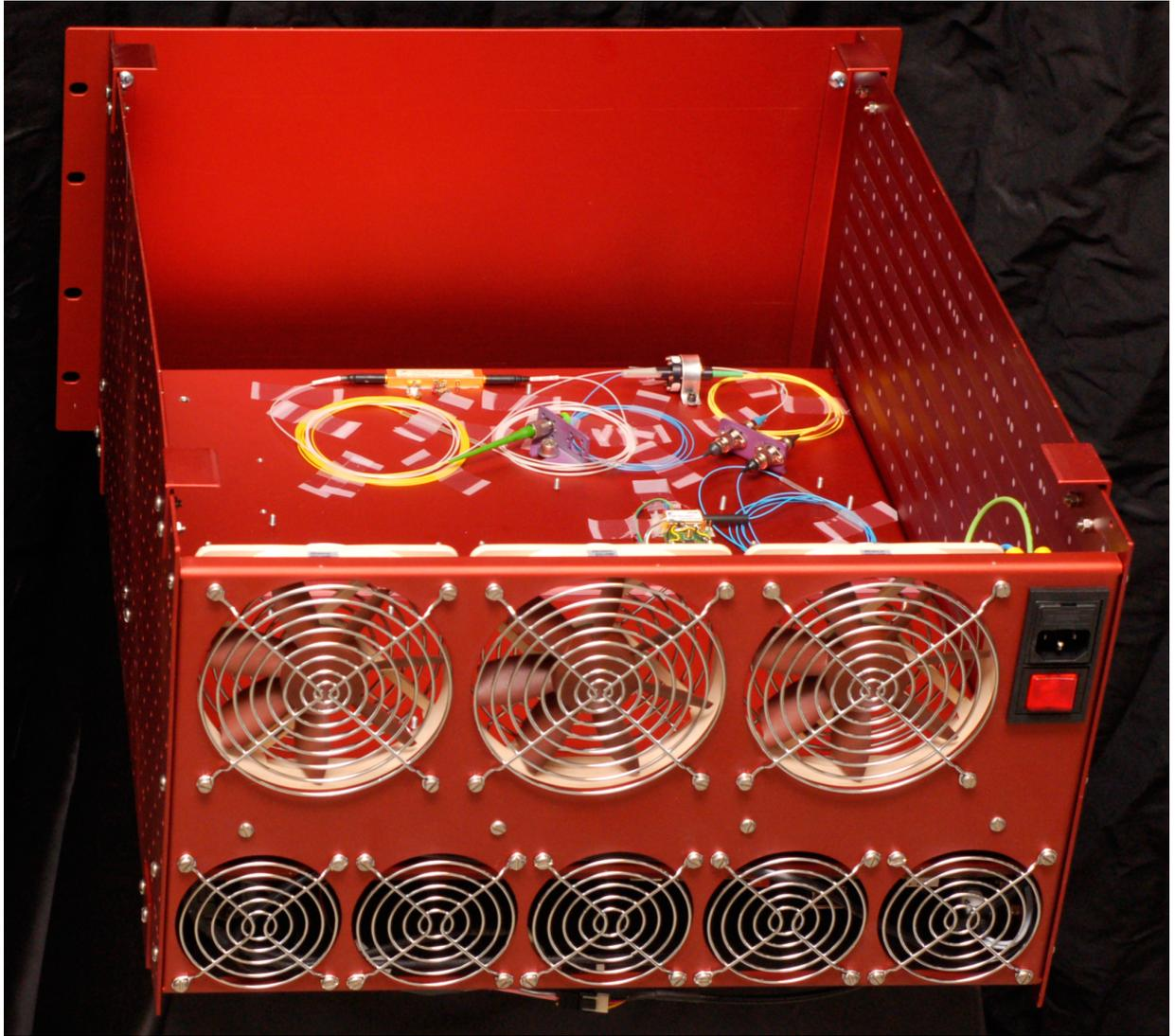
Figure 4.2: Alice's rack case. Back side view, with optics shown.
