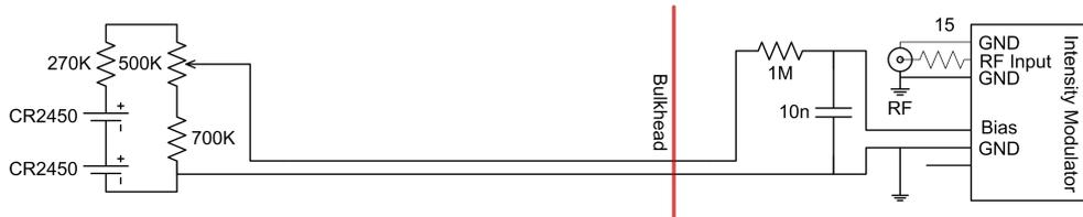
Figure 3.7: Intensity modulator biasing circuit
