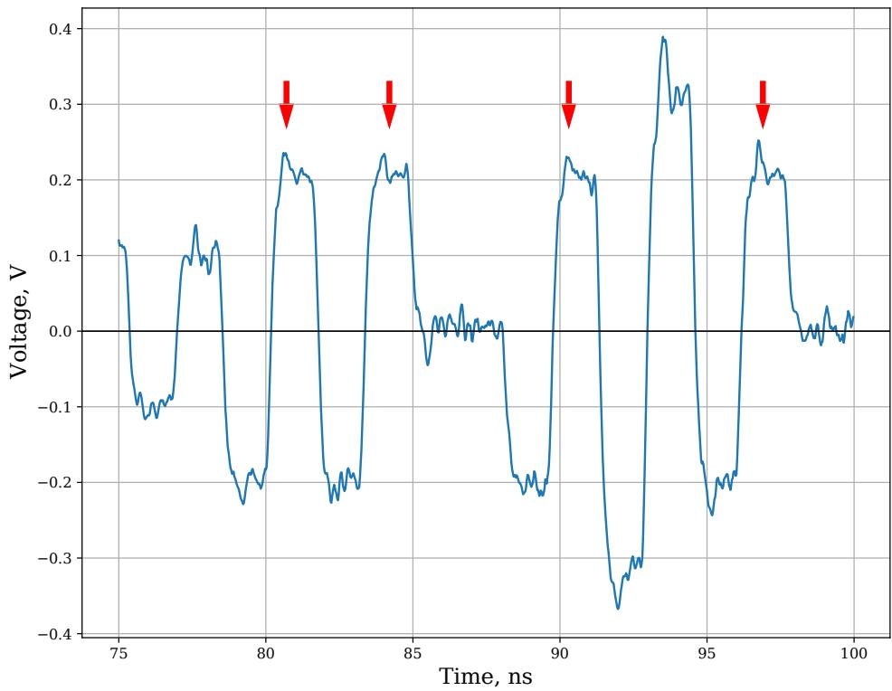
Figure 3.6: A fragment of the PM electrical signals measured oscillosogram. Red arrows denote the possible correlation effects of the same signal state (in this case, a decoy state).
