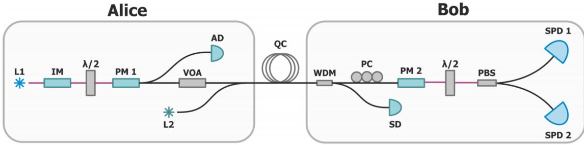
Figure 2.1: Scheme of the QRate’s commercial QKD system (taken from [51], see text for details).
