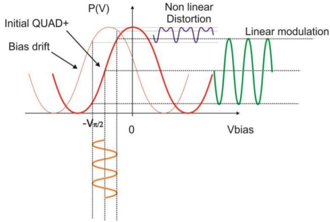
Figure 2.6: Demonstration of the transfer function drift (taken from [55]).
