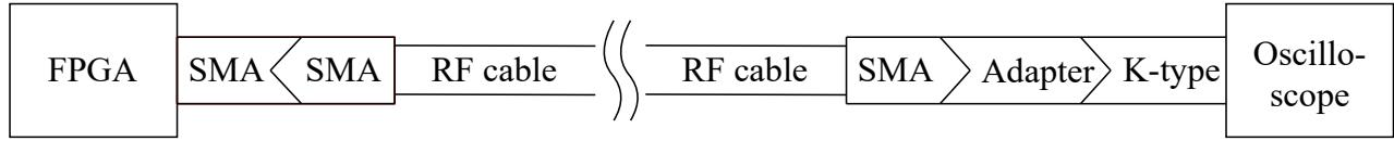
Figure 3.2: A connection between the main FPGA and the oscilloscope.
