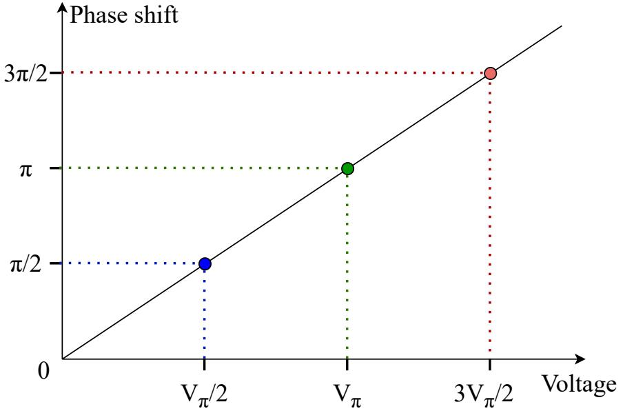
Figure 2.7: An application of the phase shift from the PM to a lightwave versus the voltage on its RF electrodes.
