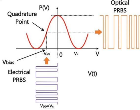
Figure 2.5: Defining the operating point on the transfer function of the IM (taken from [55]).
