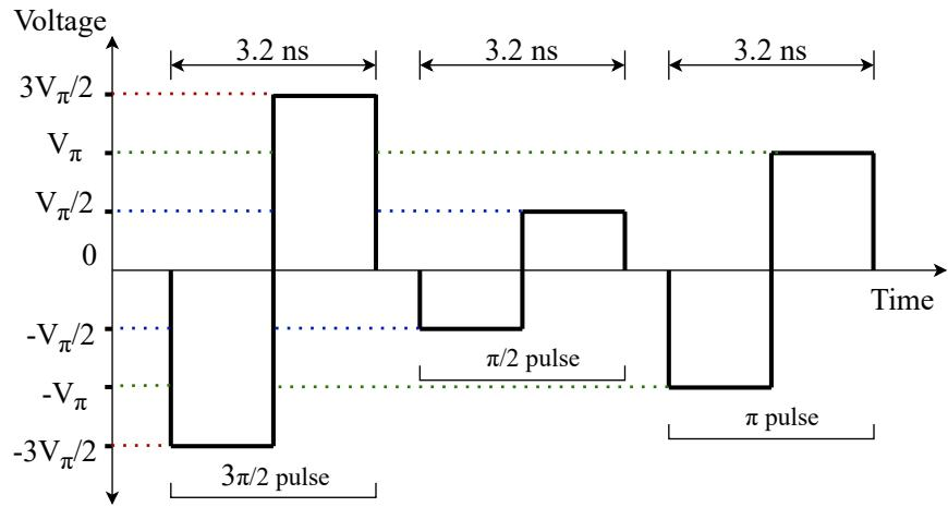
Figure 3.4: Demonstration of the all possible amplitude levels for the PM pulses.
