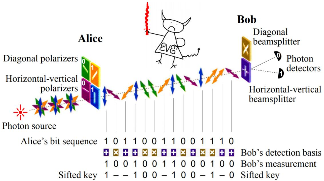
Figure 1.1: Polarization-based BB84 protocol explained (taken from [21], firstly printed in [22]).
