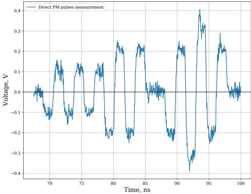
Figure 3.5: The oscillogram of the PM pulses measured directly.
