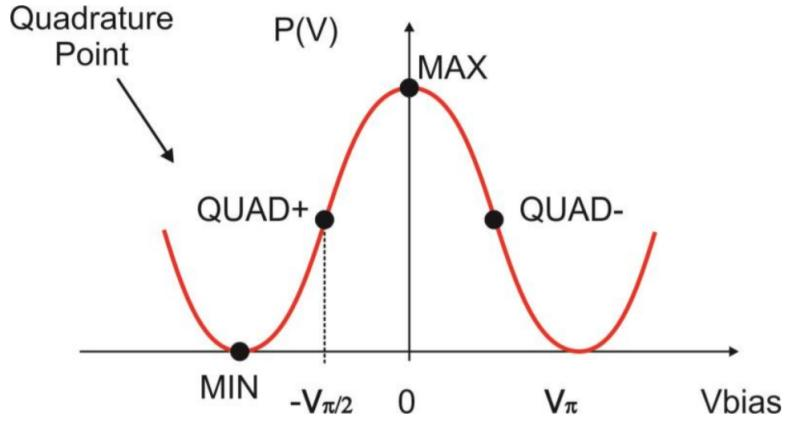
Figure 2.4: Transfer function of the IM (taken from [55]).
