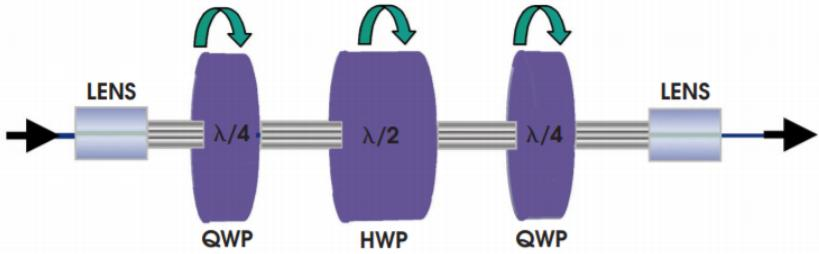
Figure 2.2:  $\lambda/4$ - $\lambda/2$ - $\lambda/4$  mechanical polarization controller (taken from [52]).
