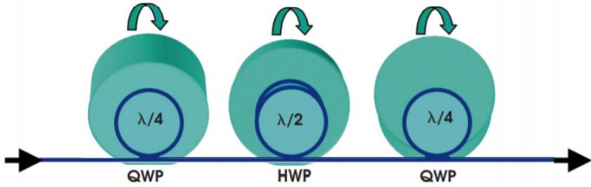
Figure 2.3:  $\lambda/4-\lambda/2-\lambda/4$  fiber polarization controller (taken from [52]).
