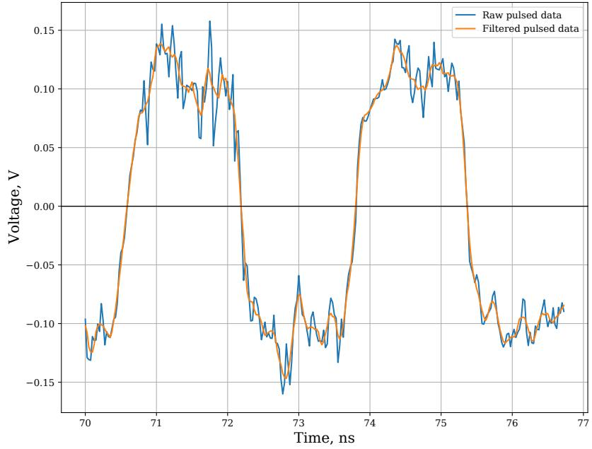
Figure 3.7: The application of digital filtering.
