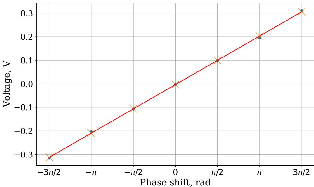
Figure 3.9: Approximation function (red) of the voltage by least squares method (measured voltage values - blue dots, approximated values - orange crosses).
