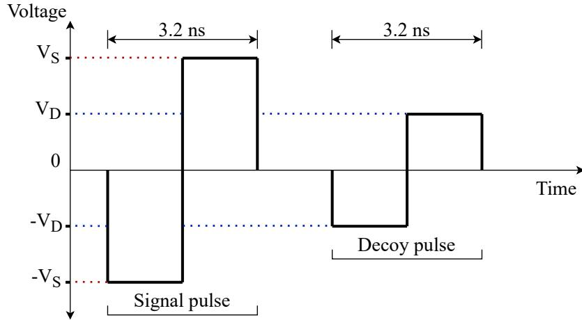
Figure 3.3: Demonstration of the signal and decoy pulses.
