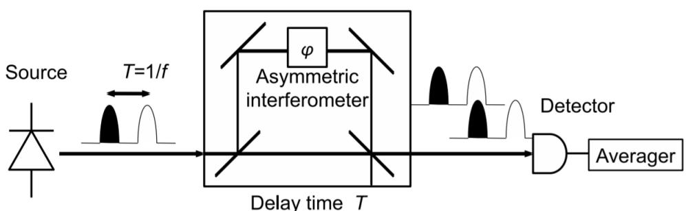
Figure 4.1: A schematic diagram of the measurement device for the correlations in the phase of the adjacent optical pulses (taken from [45]).
