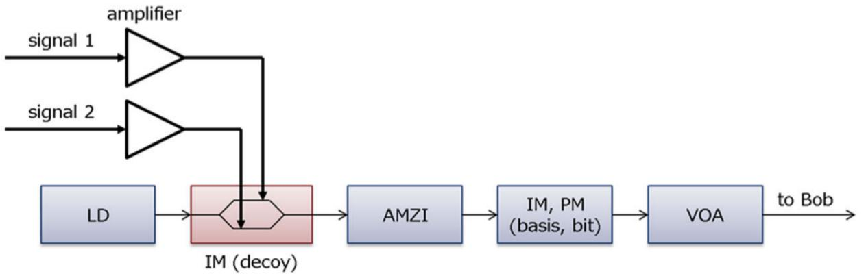
Figure 4.2: A schematic diagram of the measurement device for the correlations in the intensity of the adjacent optical pulses (taken from [50]). LD - laser diode, AMZI - asymmetric Mach-Zehnder interferometer, IM - intensity modulator, PM - phase modulator, VOA - variable optical attenuator.
