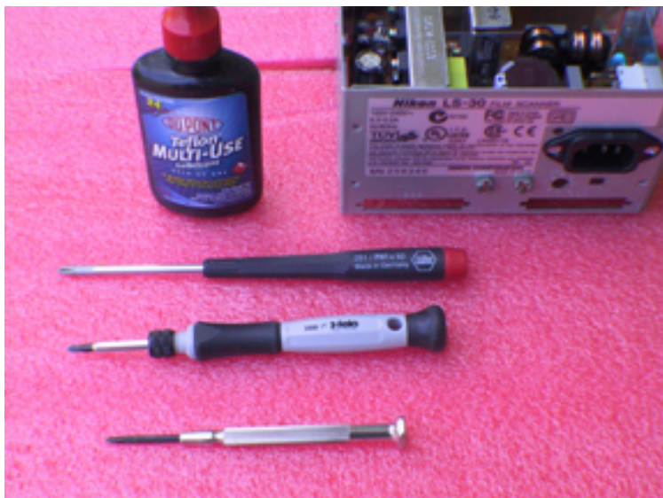
Fig 1. Jewelers screwdrivers, typical Radio Shack in front, Felo Phillips #0 with hex shaft middle, and Wiha Phillips #1 in back, with Teflon lubricant
