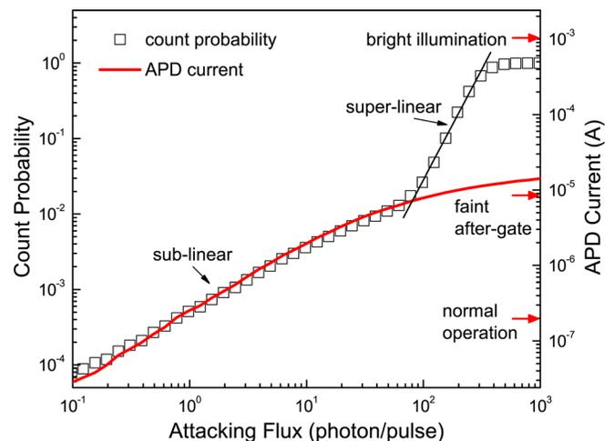
FIG. 1. (Color online) Count probability and photocurrent, when under the faint after-gate attack, as a function of photon flux. Arrows in the right axis label respective currents measured for normal operation, faint after-gate attack, and bright illumination attacks.
