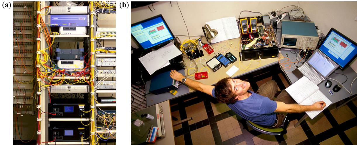
**Fig. 1.** Commercial QKD equipment vintage 2010. (a) Systems from ID Quantique installed together with high-speed classical link encryption equipment in a network node, encrypting all traffic with two other nodes. (b) A quantum hacker (L. Lydersen) at work, testing MagiQ Technologies QPN 5505 system for loopholes [5].
