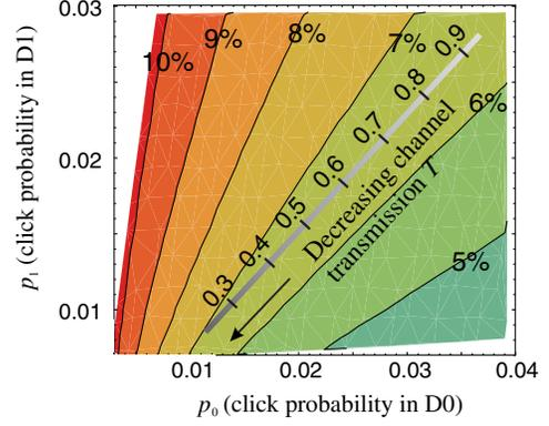
FIG. 4 (color online). Minimum QBER versus click probabilities in  $D0$  and  $D1$ . Eve minimizes the error with a suitable choice of the mean photon number of the faked states (for this plot,  $1 < \mu_0 < 100$  and  $21 < \mu_1 < 120$  at Bob's detectors). The thick shaded line indicates Bob's detection probabilities. The QBER introduced by Eve stays below 7% for  $T \geq 0.25$ .
