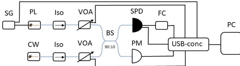
Fig.1 Experimental setup. SG – signal generator, PL – pulse laser, CW – continuous laser, Iso – isolator, VOA – variable optical attenuator, BS – beamsplitter, SPD – single-photon detector, PM – power meter, FC – frequency counter, USB-conc – USB concentrator, PC – personal computer.
