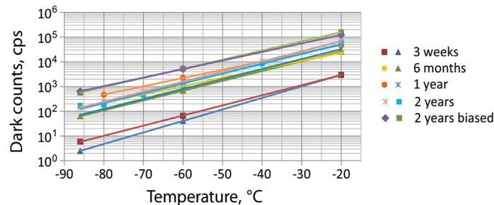
Fig. 1. The cooling effect on the measured dark count rate for SLIK APDs after various levels of irradiation (equivalent radiation time listed). Two samples were tested at each radiation level.
