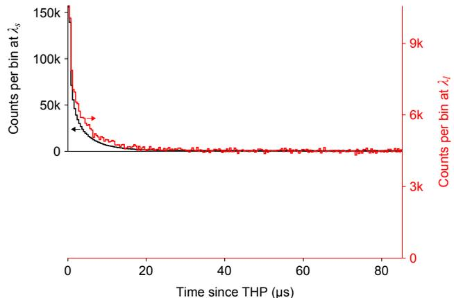
FIG. 1. Afterpulse profiles measured at  $\lambda_s = 1536$  nm and  $\lambda_l = 1924$  nm. For easier visual comparison, the histograms are rescaled so that their peak counts and dark count rates match in the plot.
