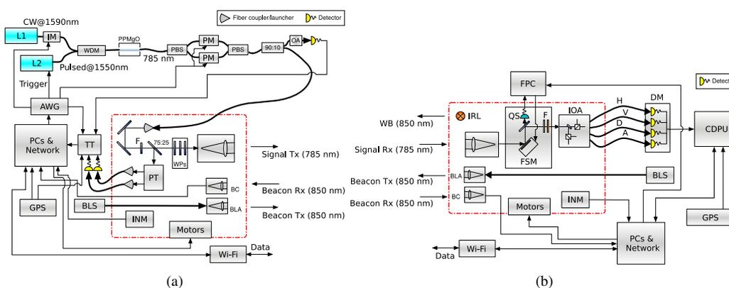
Fig. 1: Schematic diagrams of (a) the transmitter and (b) the receiver. Most receiver subsystems are custom designed and have clear path to flight.
