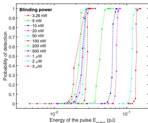
FIG. 1. Probability to force a detection as a function of the trigger energy for an NFAD.
