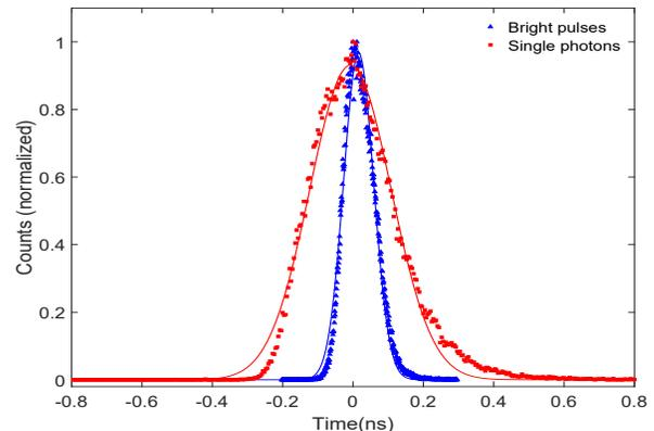
FIG. 2. Time Jitter for bright pulse and single-photons for an NFAD. Bright pulse jitter is 100.6 ps full-width-half-maximum (FWHM), while it is 271.8 ps FWHM for single photons.
