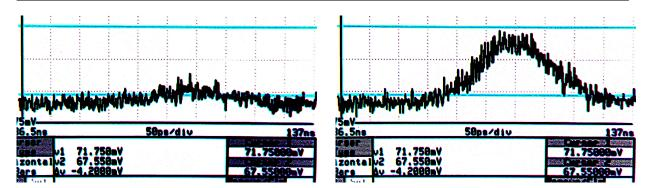
Figure 5.10: Destructive and constructive interference of output one.
