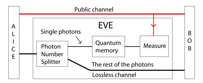
Figure 2.3: Photon number splitting attack
