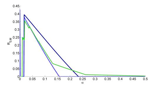
Figure 3.2: Key generation rate plot with erroneous estimate of  $\delta_{ph}$ . Maximum allowed iteration is 100. For plot guide see caption of figure 4.6.
