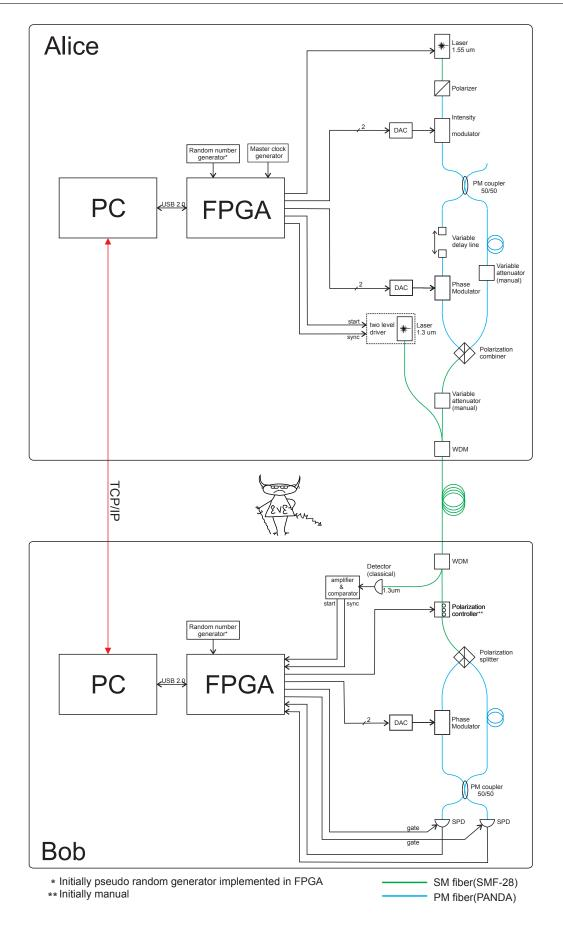
Figure 5.1: Planned structure of the QKD system. This is an updated version of the one drawn by [29].
