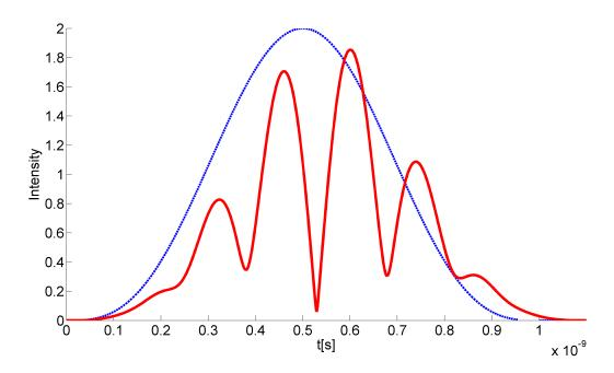
Figure 5.7: Fringes caused by time delay and varying wavelength. The frequency starts at 200 THz (1.5  $\mu$ m) and increases as a function of time. The blue dashed curve corresponds to zero time delay. The red solid curve, where fringes appear, correspond to a 0.1 ns time delay. The fringes are 700 MHz, which is the same as the delay induced frequency difference.
