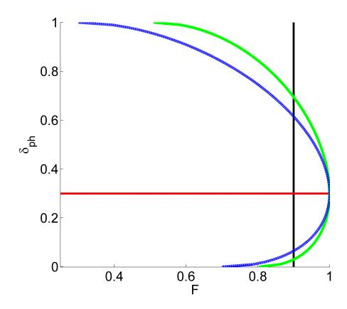
Figure 2.4:  $\delta_{ph}$  (curved) for equation (2.23) (blue dashed) and equation (2.24) (green solid) as a function of fidelity with  $\delta_1 = 0.3$  (red vertical). Two solutions of  $\delta_{ph}$  (black vertical) are possible.
