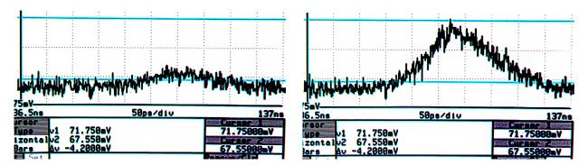
Figure 5.11: Destructive and constructive interference of output two.
