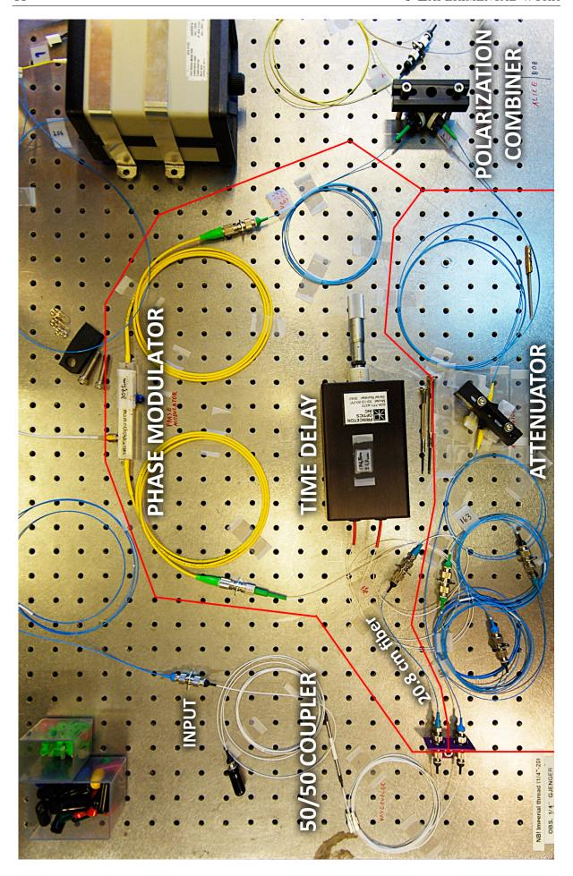
Figure 5.13: Alice's part of the interferometer
