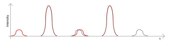
Figure 5.5: Subsequent pulses with proper time delay
