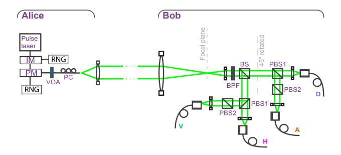
Figure 3.1: Polarization encoding free-space BB84 system (reprinted from [1]).
