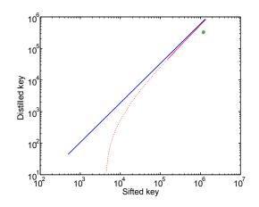
FIG. 3. Experiment result with the new software. Blue line is the infinite key bound. Red-dotted line is finite-key size bound with  $\epsilon = 10^{-10}$ . Green stars are experiment results
