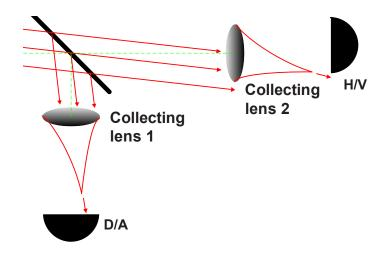
Figure 4.2: An illustration of spatial-mode detection efficiency mismatch. The beam from Eve (red line) is sent to Bob in an angle diverging from the normal setup by Alice and Bob(green line). This angle is picked such that the beam path hit the collecting lens 1 and being detected in the D/A basis, but misses the H/V detector. Thus, this angle can be used to send D/A fake state to Bob without inducing error(modified from [55]).
