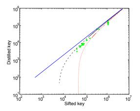
FIG. 2. Secret key rate vs raw key rate. Blue dashed line is the infinite key bound. Red dotted line is finite-key size bound with  $\epsilon = 10^{-10}$ . Black line is finite-key size bound with  $\epsilon = 10^{-1}$ . Green dots are experimental result with 3 dB line loss and 5.2% error rate.
