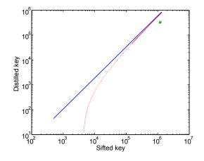
Figure 4.11: Experiment result with the new software. Blue line is the infinite key bound. Red-dotted line is finite-key size bound with  $\epsilon = 10^{-10}$ . Green  $\times$  are experiment results.
