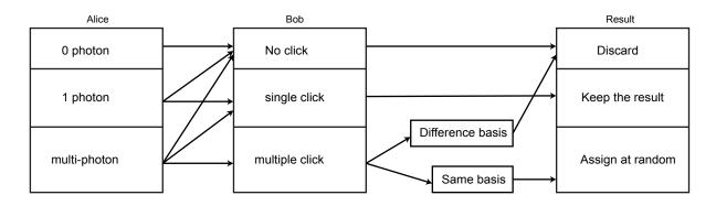
Figure 3.3: Squashing model for BB84 system. (reprinted from [13])
