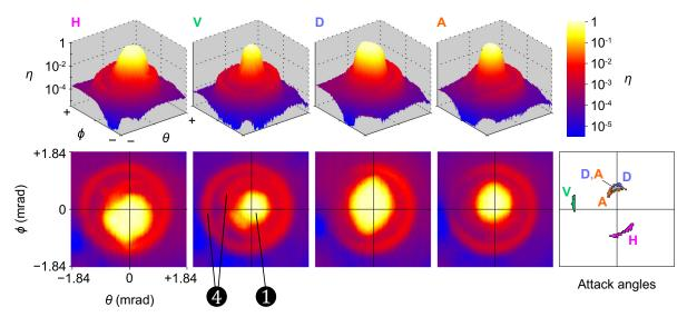
FIG. 2. (Color online) Angular efficiency scan of the receiver, and points of interest. Four pairs of plots **H**, **V**, **D**, **A** shown in both three-dimensions and two dimensions represent normalized detection efficiency in the four receiver channels versus illuminating beam angle  $(\phi, \theta)$ . The angle  $\phi = \theta = 0$  is the initial angle of QKD operation. The last plot shows angle ranges with a high mismatch, which is usable in our attack.
