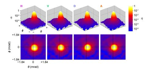
Figure 4.6: Angular efficiency scan of the receiver after a 25 µm diameter pinhole (Thorlabs P25S) is placed in the focal plane of L1, L2 [4.3(a)]. No detectable mismatch between channels was found under tight search conditions  $\eta_i(j) \ge 0.001$  and  $\delta_i(j) \ge 4$ .
