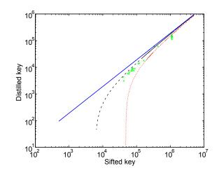
Figure 4.10: Secret key rate vs raw key rate. Blue dashed line is the infinite key bound. Red dotted line is finite-key size bound with  $\epsilon = 10^{-10}$ . Black-line is finite-key-size bound with  $\epsilon = 10^{-1}$ . Green dots are experimental results with 3 dB line loss and 5.2% error rate.
