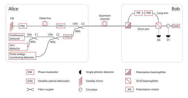
Figure 3.2: Plug-and-play system. Reprinted from [13]
