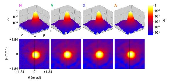
FIG. 4. (Color online) Angular efficiency scan of the receiver after a 25- $\mu$ m-diameter pinhole (Thorlabs P25S) is placed in the focal plane of L1, L2 [Fig. 1(a)]. No detectable mismatch between channels was found under tight search conditions  $\eta_i(j) \ge 0.001$  and  $\delta_i(j) \ge 4$ .
