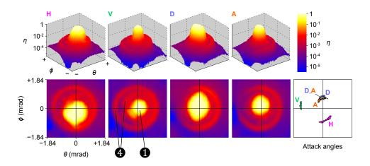
Figure 4.4: Angular efficiency scan of the receiver, and points of interest. Four pair of plots **H**, **V**, **D**, **A** shown in both 3D and 2D represent normalized detection efficiency in the four receiver channels versus illuminating beam angle  $(\phi, \theta)$ . The angle  $\phi = \theta = 0$  is the initial angle of QKD operation. The last plot shows angle ranges with a high mismatch, usable in our attack.
