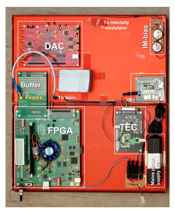
Figure 4.3: Electronic side of the bulkhead
